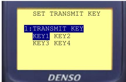
Use the Cursor keys to select the appropriate key then press the **C** key. The screen will prompt "Set up? 1:Yes **2:No**". If the new Key is correct press **1 ENT** to return to the SECURITY CONFIG menu.
